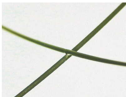
0.01" diameter tungsten cross wire weld
