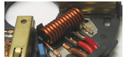
Terminal connections for sensors
