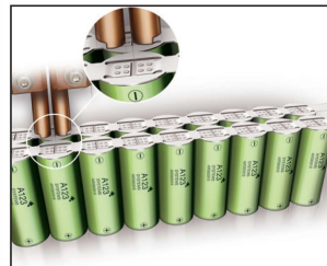
Battery pack welding
