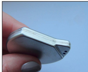
Seam Welding of pacemaker cases
