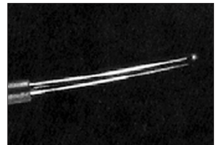
(3) Remove welded thermocouple
