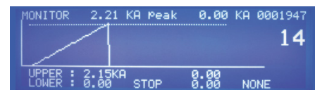
Monitor Screen – Shows weld current exceeding limit.
