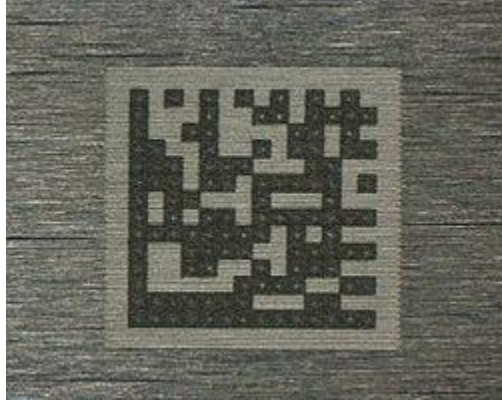
Clear 2D marking on aluminum.
